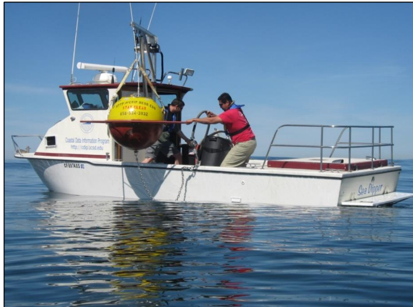
Figure 2-3. CDIP personnel deploy a Datawell directional Waverider. As of 2015, the CDIP network is composed of approximately 60 wave observation sites. (Photo courtesy of SIO/CDIP)
