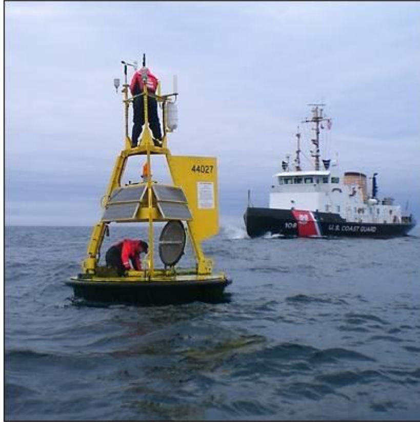
Figure 2-2. NDBC 3-m discus buoy being serviced at sea from U.S. Coast Guard vessel. (Photo courtesy of Richard Bouchard/NDBC)
