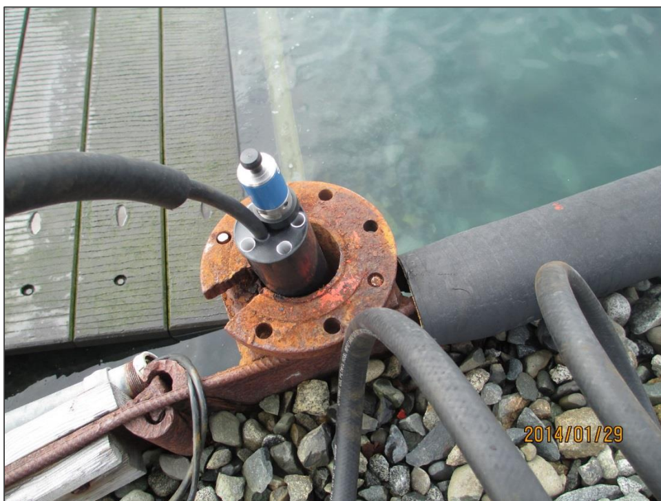
Figure 2-5. An Aanderaa 5218 pressure sensor is lowered into a protective well, providing single point, non-directional wave observations. (Photo courtesy of Richard Butler/Aanderaa)
